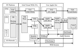
Figure 2. Three-layer security model of the VWSS-UC.
