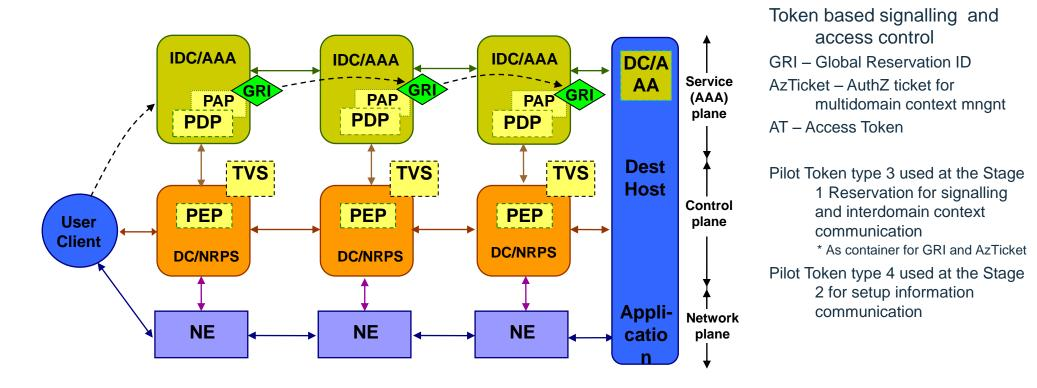
IDC – Interdomain Controller DC – Domain Controller NRPS – Network Resource Provisioning System NE - Network Element
