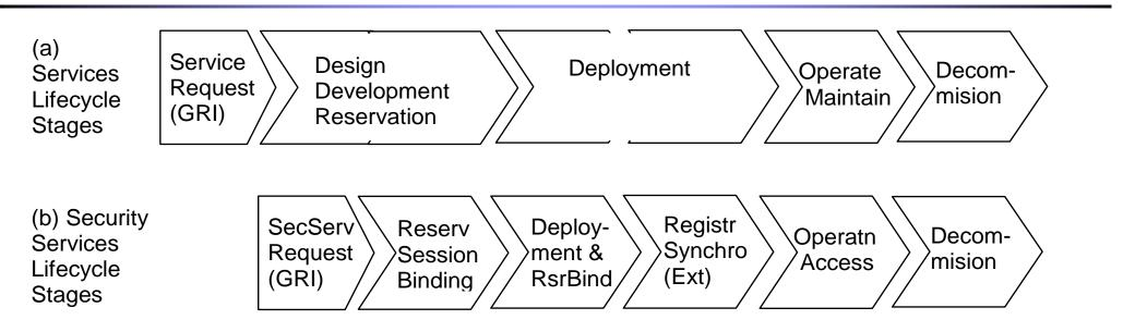
Additional SSLM stages and mechanisms to ensure consistency of the security context management Security Service Request that initiates creation of the dynamic security association and may use SLA security context.
