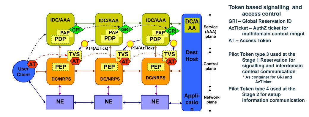
IDC – Interdomain Controller DC – Domain Controller NRPS – Network Resource Provisioning System NE - Network Element
