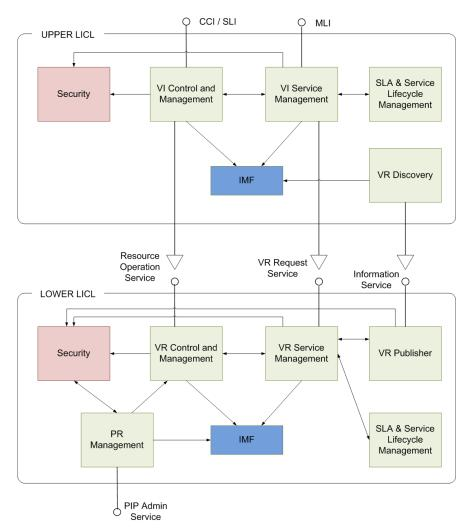
Figure 2.3?: LICL functional architecture overview
