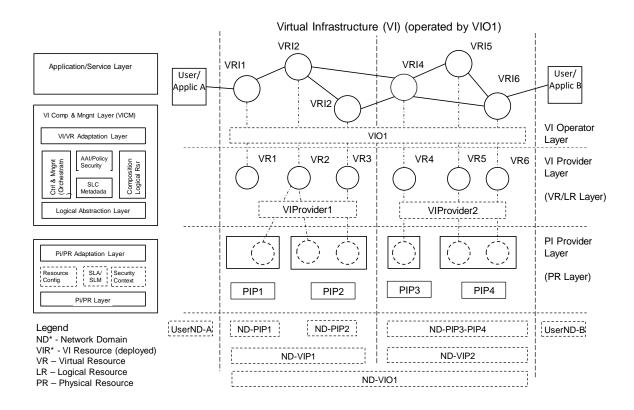
Figure 2.3. Main actors, functional layers and processes in on-demand infrastructure services provisioning
