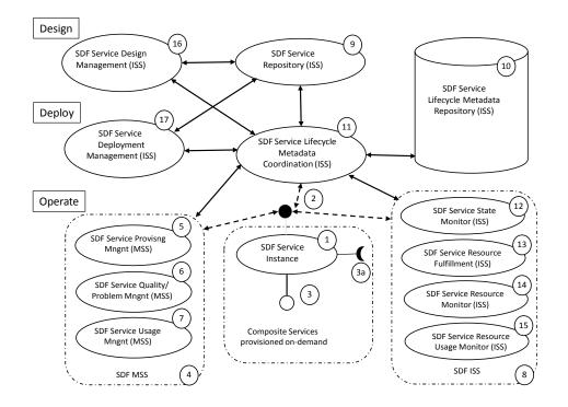
Figure C.2. SDF main components and their interaction during Design, Deployment and Operation Stages
