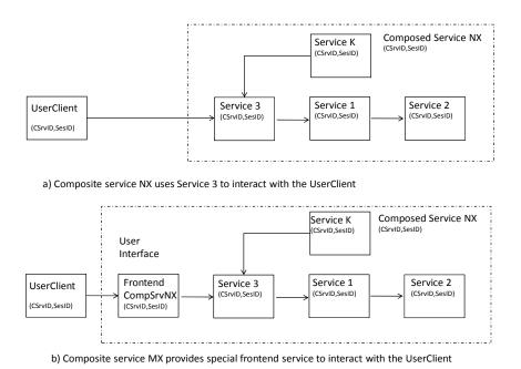
Figure 11. Example composite service composed of services Service 1, Service 2, Service 3, Service 4.
