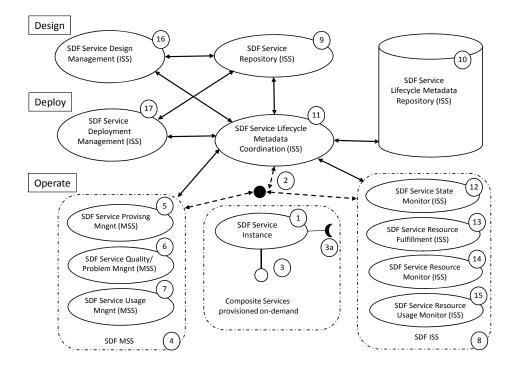
*Figure A.2. SDF main components and their interaction during Design, Deployment and Operation Stages*
